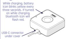
First, charge your device using the charging cord behind the case insert. You can use the device while it's charging, Full charge will be reached after 3 hours and battery light will turn solid green.
